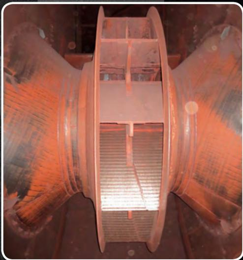
**Clarage's New Impeller After 18 Months of Operation with no wear**
