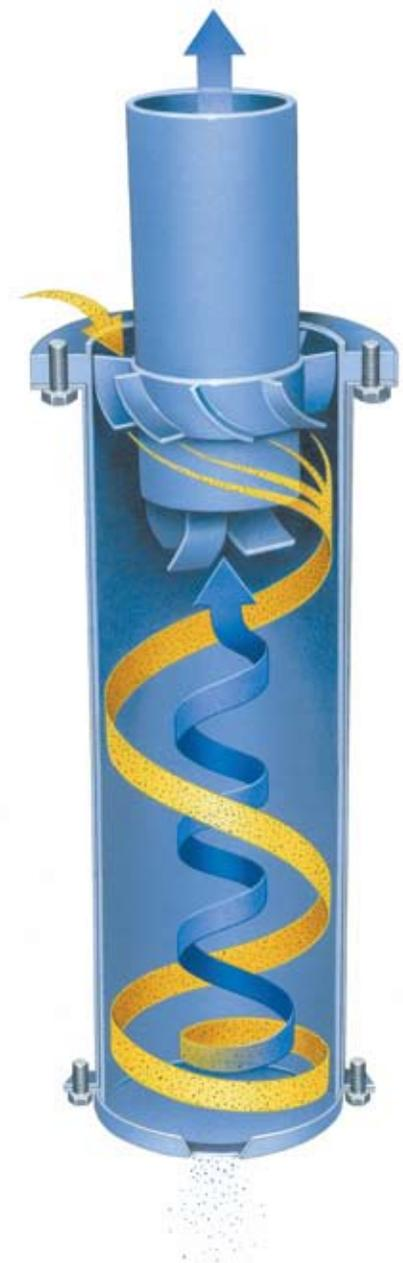
Operation of collecting tube assembly.
