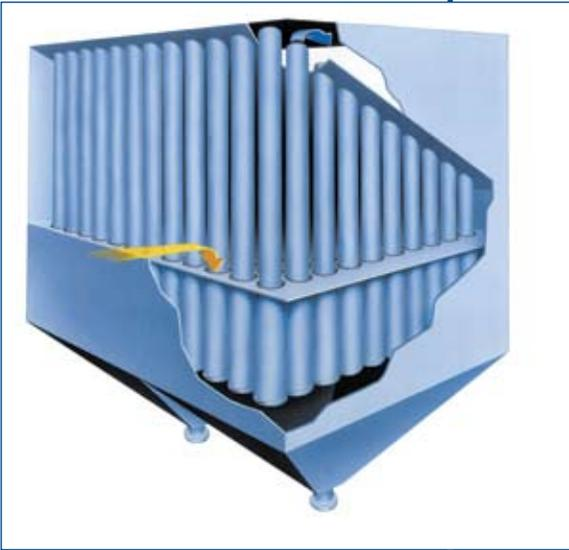
The STD design collector is most commonly used in smaller industrial applications. The greatest advantage of the STD collector is its compact design that can easily accommodate space limitations. Additional advantages of the STD collector design can be realized through cost reduction in insulation and lagging area, as well as a smaller support structure.
