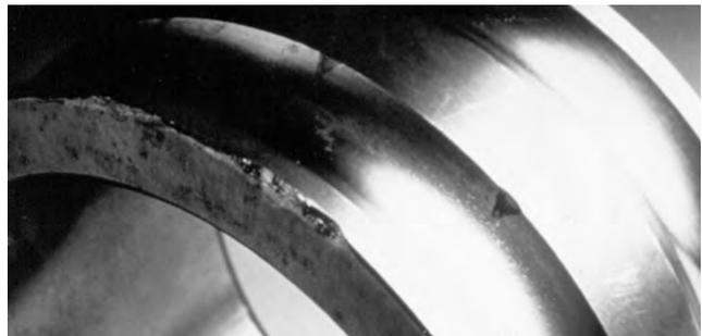
failures. Figure 22 shows the surface of a bearing bore that had too much clearance. The shaft turned in the bore, smearing the surface.
