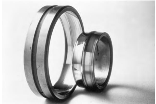
unloaded to being under load. With the light load it takes them some distance to roll properly, and they skid against the race causing smearing.
