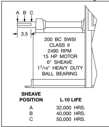
Figure 2. Effect of Sheave Diameter on Bearing Life
