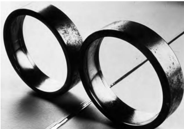
Figure 22. Smearing on a Bearing Race
