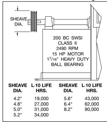
Figure 3. Effect of Shaft Position on Bearing Life
