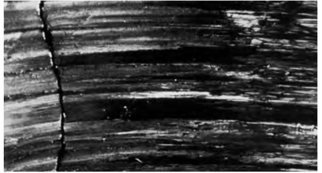
Figure 23. Fretting Corrosion on Bearing Bore
