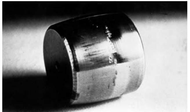
Allowing electrical current to pass through a bearing can cause damage. Figure 26 shows a spherical roller with pits in its surface caused by electrical current. This type of damage commonly occurs when welding balance weights on a fan wheel with improper grounding. To avoid having the welding electrical current pass through the bearings, attach the grounding clamp to the wheel or shaft when adding balance weights.
