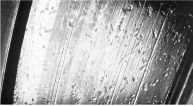
probably due to seal failure, possibly in a “wash down” environment. High moisture applications require the use of grease that has rust inhibiting properties. Frequent relubrication is necessary, to insure that all bearing surfaces are coated with a protective layer of grease and that the rust inhibitors are replenished. Figure 15 shows a spherical roller bearing roller that has rusty ends from moisture in the lubricant.
