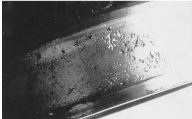
wear due to inadequate lubrication. The rollers have worn a very deep wear pattern in the race.
