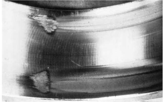
Figure 12. Highly Polished Surfaces Due to Inadequate Lubrication
