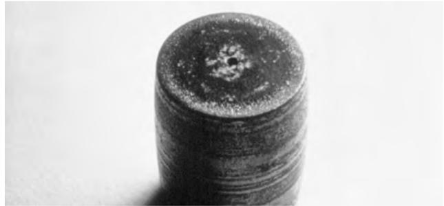
Figure 16. Puddle Corrosion
