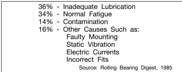
If bearings that are failing can be taken out of service before they are completely destroyed, they can reveal information about the cause of failure. Different modes of failure leave unique evidence in the bearing components. The rest of this article shows how the more common types of fan bearing failures affect bearing components.
