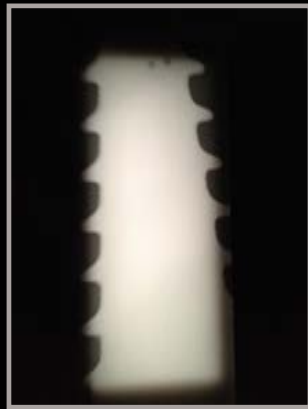
X-RAY OF HOLDING PATTERN (OLD SHAFT)
