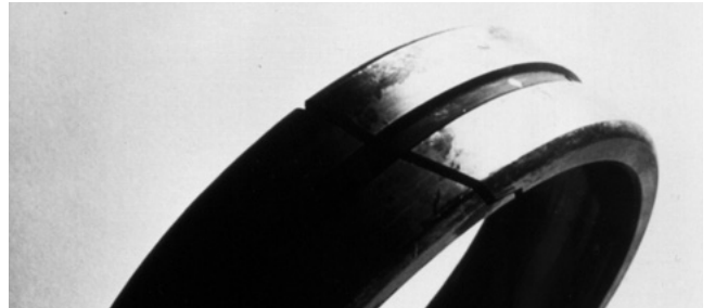
Figure 26. Pits Caused by Electrical Current
