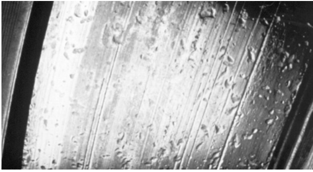
Figure 13. Severe Particle Denting
