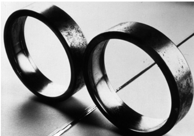
Figure 21. Two Load Zones on the Outer Race
