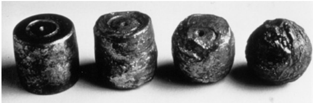
Figure 9. Damaged Spherical Bearing Rollers
