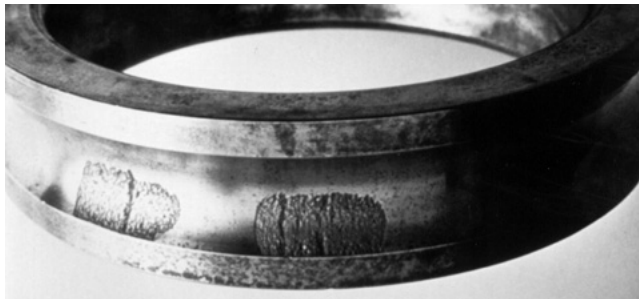
Figure 21. Two Load Zones on the Outer Race
