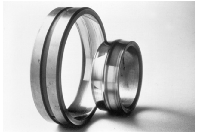
Figure 12. Highly Polished Surfaces Due to Inadequate Lubrication
