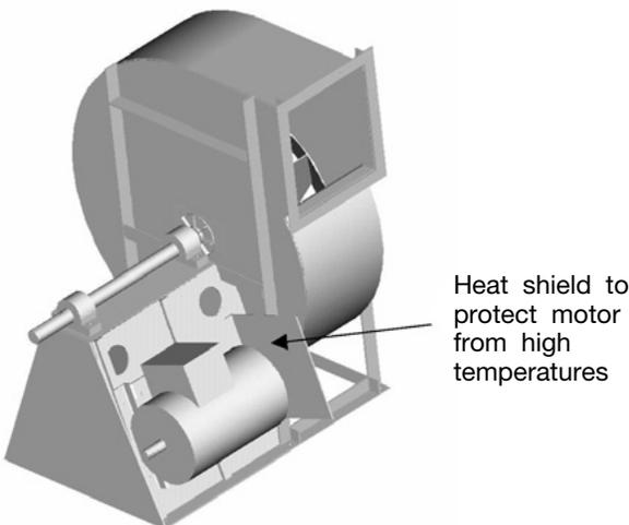
On Arrangement 10 fans, a heat shield is also used but is slightly different from the one used on an Arrangement 9 fan. Because an Arrangement 10 fan has the motor under the pedestal, the radiant heat cannot just be deflected. Therefore, it is recommended to add some insulation between the fan housing and the pedestal. See Figure 3 below.
