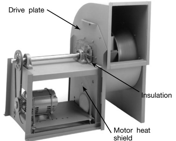
When the temperature exceeds 800°F, it is necessary to separate the pedestal from the fan housing. By doing this, the amount of heat conducted through the pedestal and to the bearings and motor is greatly reduced. The pedestal is separated from the fan by welding either a channel or angle supports between the two as shown in Figure 4.
