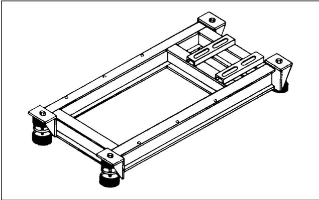
**2. Vibration Isolation Rails** — Vibration isolation rails are sometimes employed in much the same capacity as the vibration isolation base, usually on smaller arrangement 9, 10 or 4 fans. They add stiffness to the mounting platform of the fan, and height saving brackets may be used if height needs to be kept to a minimum (see Figure 3).
