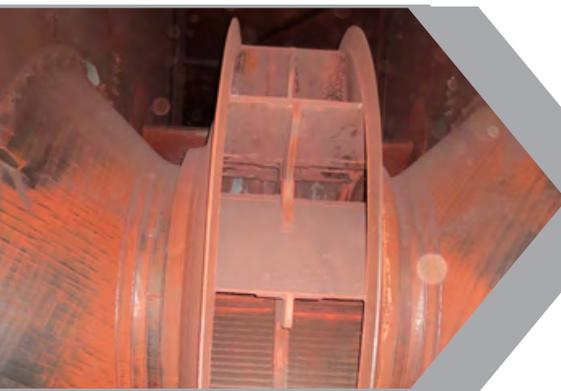
CLARAGE'S NEW IMPELLER AFTER 18 MONTHS OF OPERATION WITH NO WEAR
