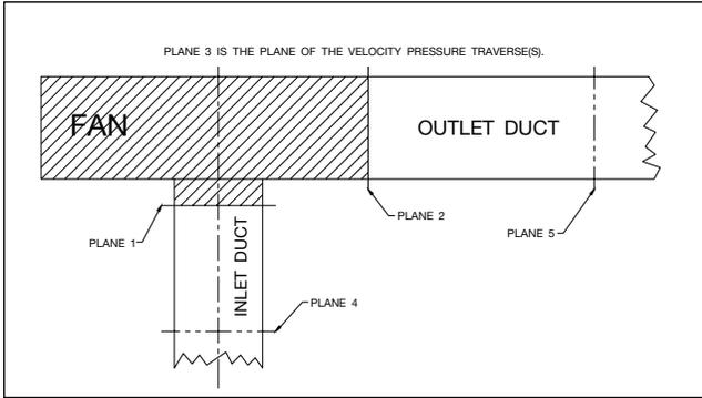
If the fan and system check out, begin testing the fan. There are five critical measurement groups that must be made to get the most accurate air performance test:
