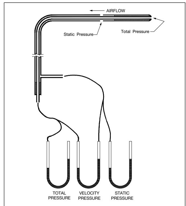
are usually very small, so they can easily become blocked in dirty or wet flows. In those situations, periodically check the tube to make sure the holes are not blocked, or use an alternate instrument for traverse measurements.
