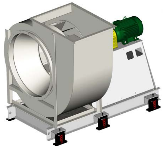
Fan mounted on an inertia base. Base and pedestal shown filled with reinforced concrete.
